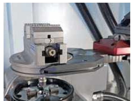
Mechanischer Zentrischspanner MZQ 170-60 PA, Erowa ITS 148 Mechanical centre-clamping vise MZQ 170-60 PA, Erowa ITS 148
