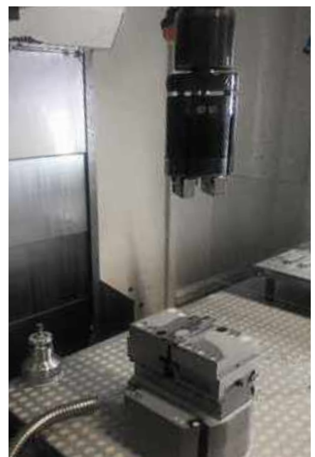
Pneumatischer Zentrischspanner PZS 180-80 AT Pneumatic centre-clamping vise PZS 180-80 AT
